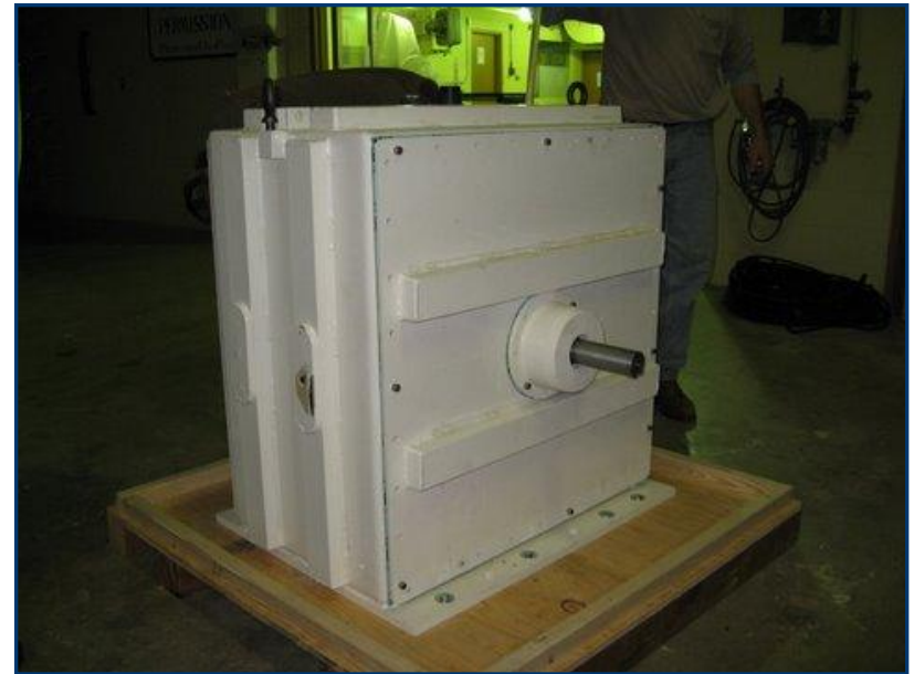
Our Underwater Permanent Magnet Generator
